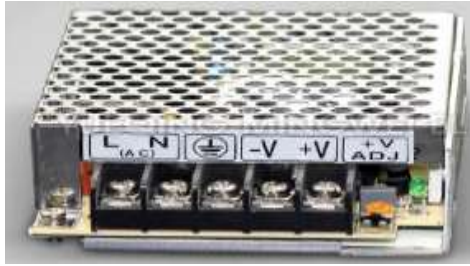
Figure19: External View of SMPS
