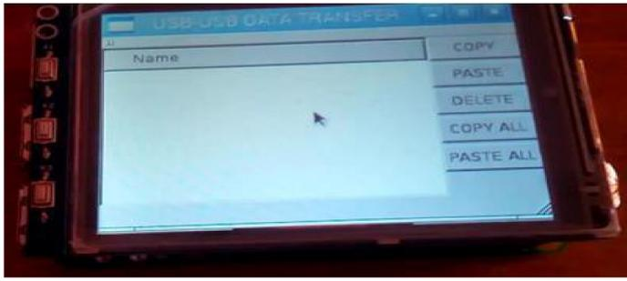
Fig.6 Display showing delete, paste, copy all, and Paste all options.
