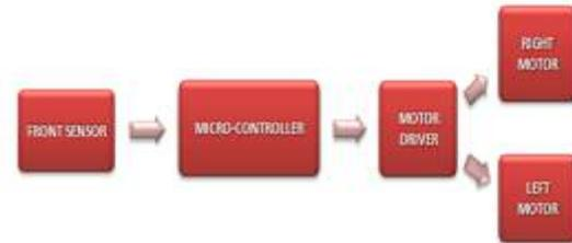
Fig 4.1: Block diagram of I won't fall down robot
