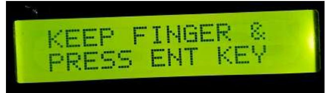
Fig 2: LCD display showing waiting for thumb print
