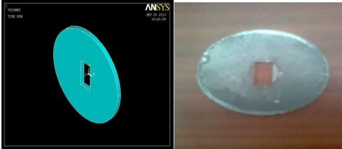
**Figure 3.7** An artistic view and a photograph showing rectangular orifice.
