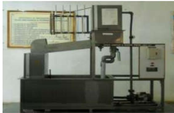
Figure 3.1 Orifice tank
