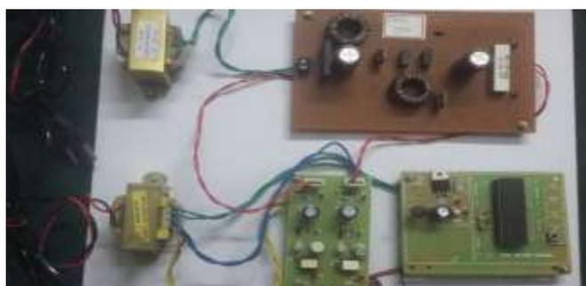
**Fig.8 Prototype of the proposed ZVT ZCT PWM converter**
