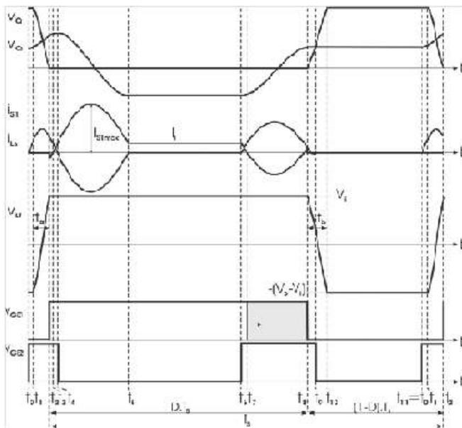
Fig.3 Timing diagram and key waveforms of the converter
