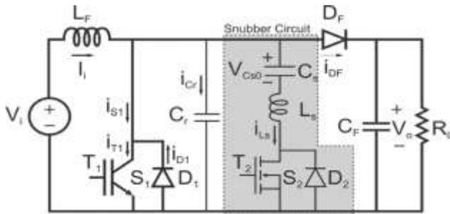
Fig.1 Circuit diagram of ZVT-ZCT-PWM boost converter.
