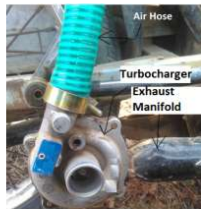
Fig 3 Installation of Turbocharger.
