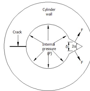
**Fig. 2: Elasto-plastic Failure**
