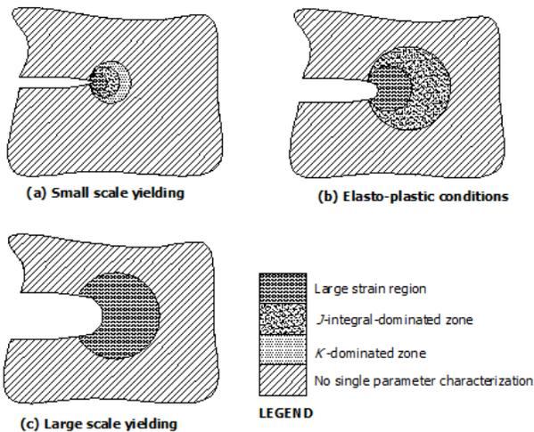
**Fig. 1: Effect of material plasticity**
