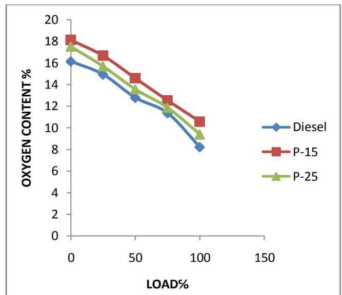
Figure (7) Variation of oxygen content with load.
