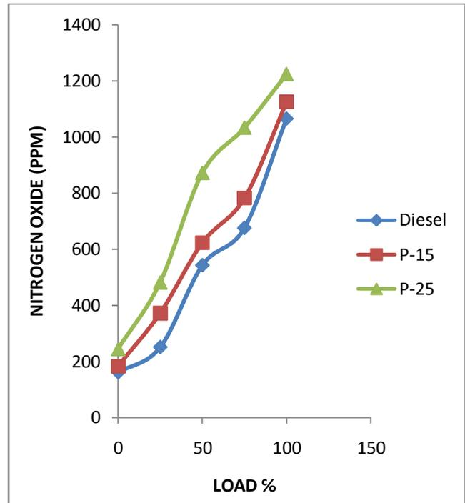
Figure (9) Variation of Nitrogen oxide emission with load
