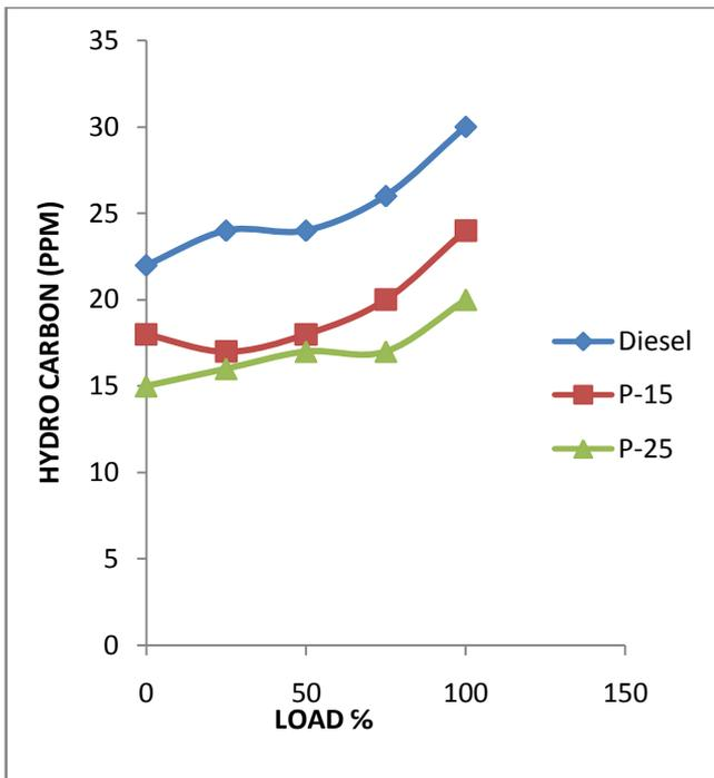
Figure (8) Variation of Hydro carbon emission with load
