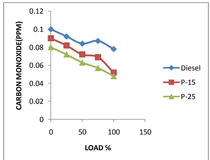
Figure (7) Variation of Carbon monoxide emission with load
