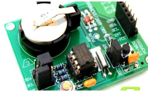
Figure 5: RTC Module
