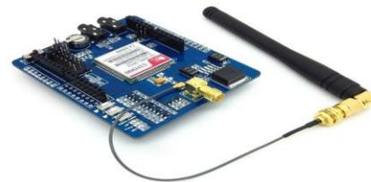
Figure 3: GSM Module
