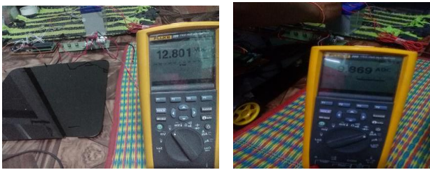
Fig. 11 DC Voltage and Ampere of Transmission Section (Distance between transmitter and receiver = 5 cm) P = VI = 12.801 \times 9.869 = 126.333 \text{ W}
