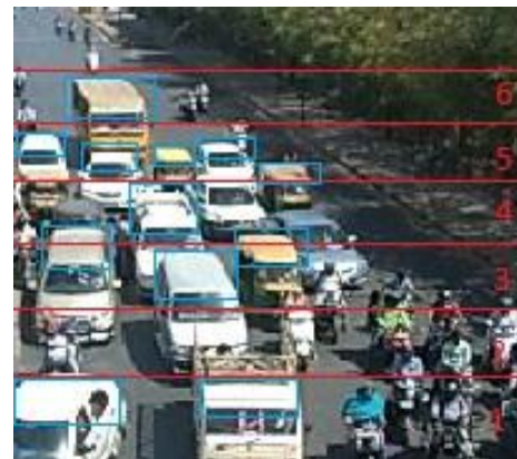
Fig. 3. Vehicle counting by calculating total number of pixel range-wise.
