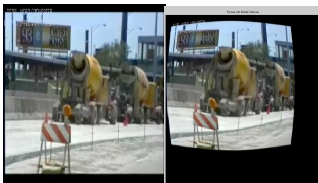
Fig. 4 Original watermarked video frame and show the effect of barrel distortion on this frame
