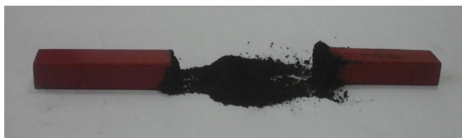
Fig. 5: Particles of iron oxide-copper ferrite-chitosan nanocomposites attracted by a bar magnet
