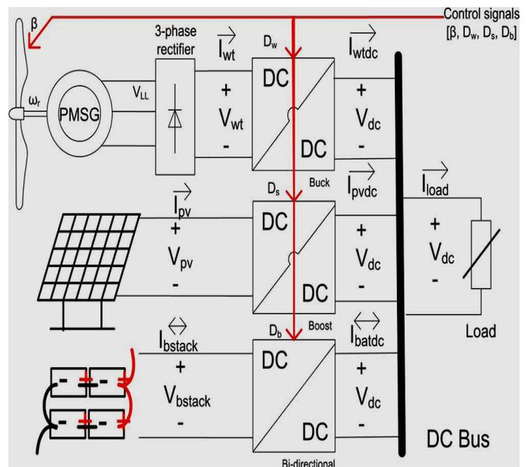
**Fig. 6.1 Topology of a Small-Scale DC Microgrid.**
