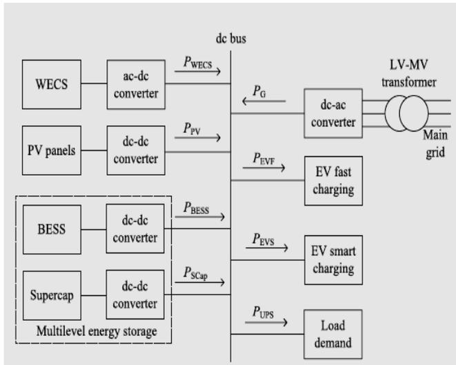
Fig. 4.1 Layout of the DC Microgrid.
