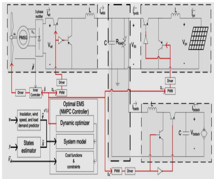
**Fig. 7.1 Simplified view of the DC Microgrid and the Developed NMPC controller. The Battery Bank is assumed to Work in Charging Mode.**
