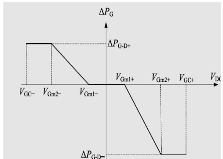
**Fig. 4.5 Droop Control of the Grid Power Electronic Converter in Interconnected Operation Mode of DC Microgrid.**
