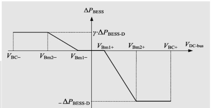
Fig. 4.3 Droop Control of BESS Power Electronic Converter to Mitigate Power
