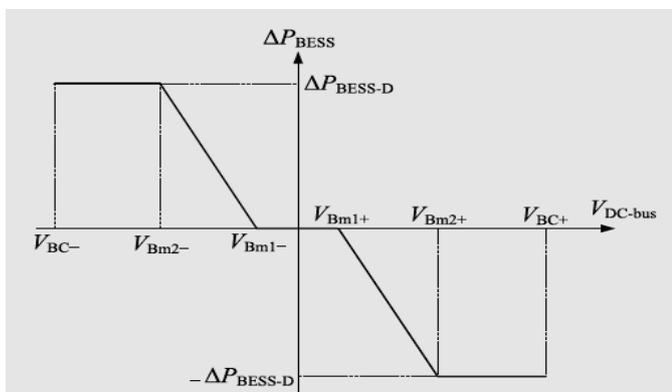
Fig. 4.2 Droop control of BESS power electronic converter to mitigate power deviations of dc microgrid in normal SOC of the BESS.
