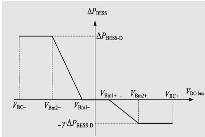
**Fig. 4.4 Droop Control of BESS Power Electronic Converter to Mitigate Power**
