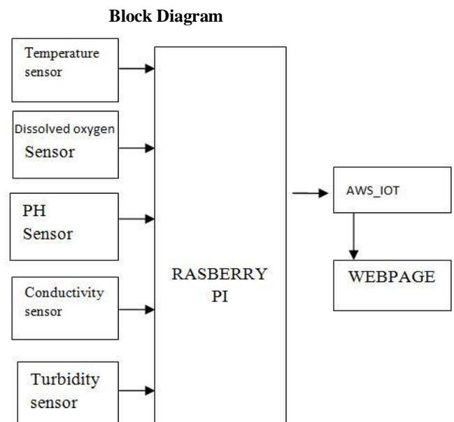
Fig.1. Water Quality Monitoring and Notification System
