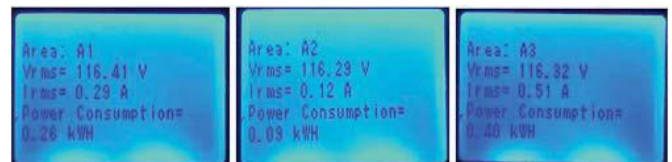
Fig.5 Energy power consumption and power parameters of different areas (a) A1, (b) A2, (c) A3
