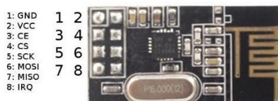
Fig. 3: nrf24L01+ pinout
