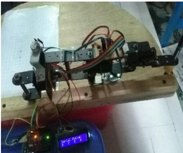
Figure.13. Testing Photo of Robot Arm Control System for Home Position ( x=30.3\text{cm} , y=0\text{ cm} and \phi=0 )
