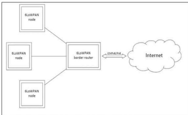
Fig. 2 Nodes and Border Router in a WPAN
