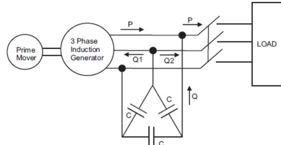
Fig.2 Schematic diagram of self-excited induction generator
