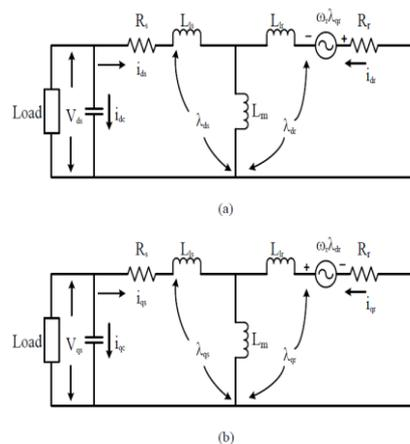
fig.4(c).Equivalent circuit of SEIG in d-q stationary reference frame (a) d-axis (b) q-axis
