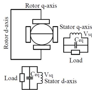
Fig.4(b).d-q axes presentation of self-excited induction generator
