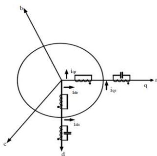
Fig.4(a).Axes transformation of induction generator
