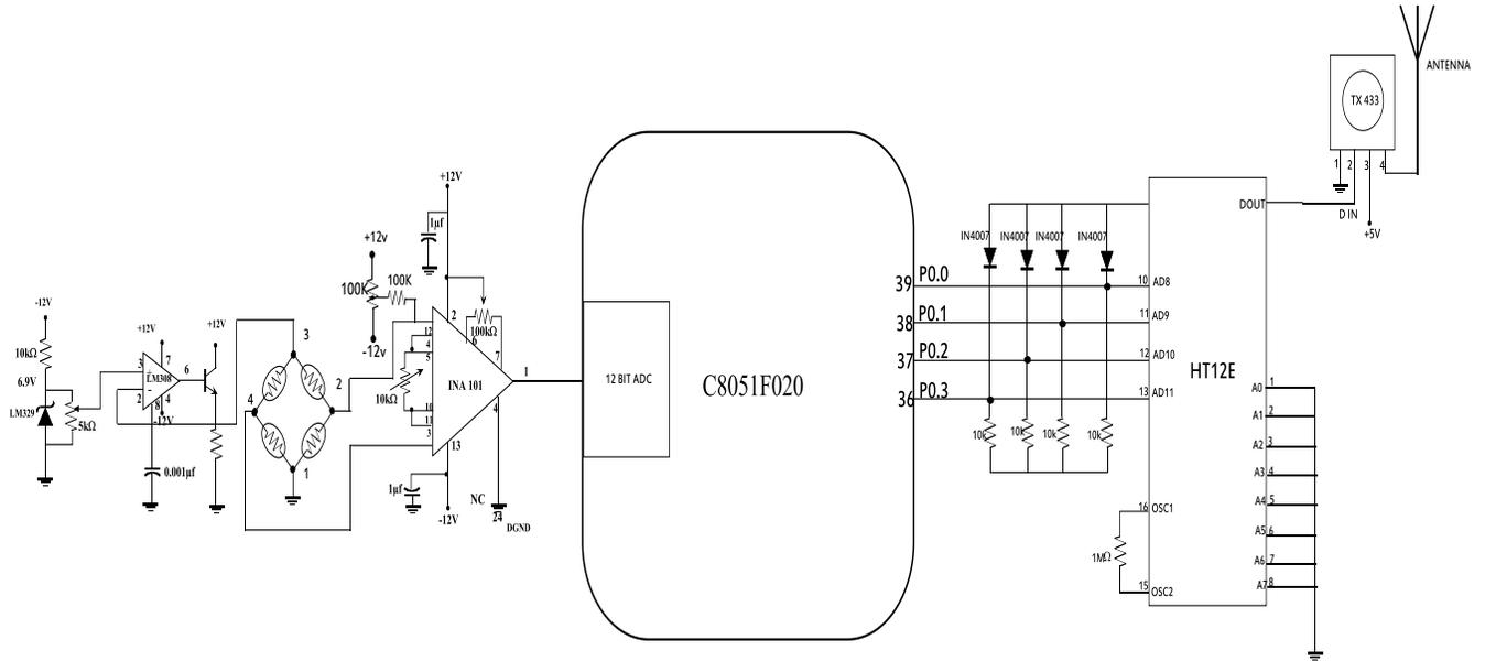
Fig 2.a Schematic diagram of Transmitting section
