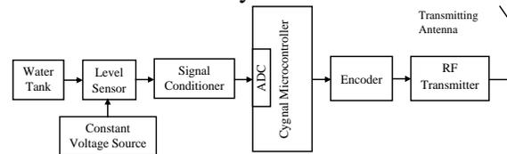
Fig. 1 Block Diagram of Transmitting Section
