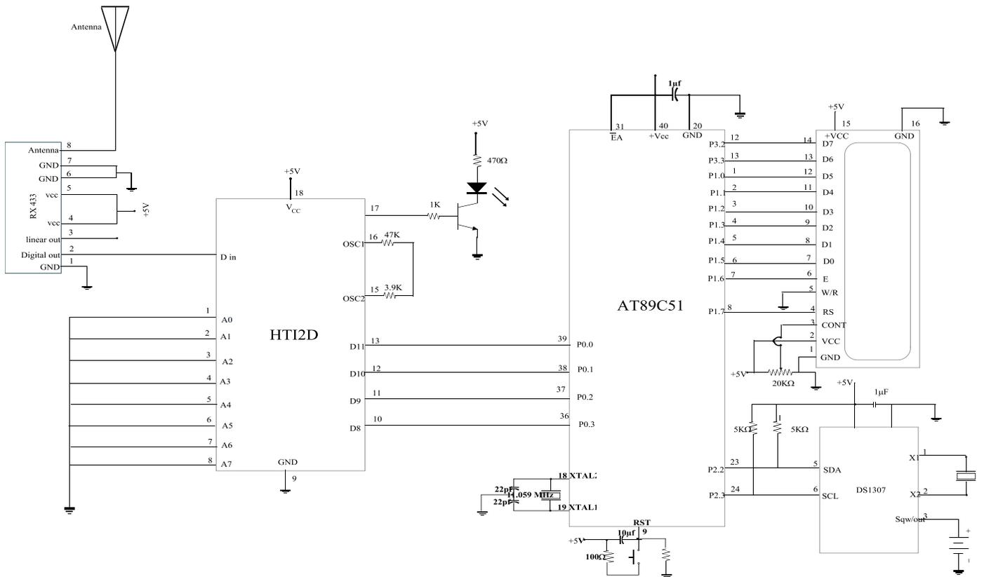
Fig 2.b Schematic diagram of Receiving section
