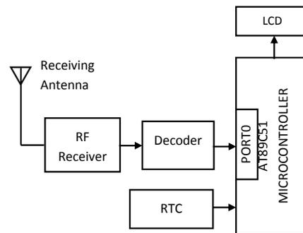
Fig. 1(b) Block Diagram of Receiving Section
