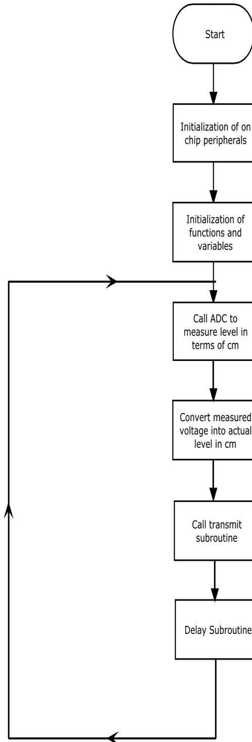
Fig 3(a) Flowchart of Transmitting Section
