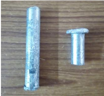
Fig. 3.2: Solidified Al 2 O 3 reinforced Al6061 composite
