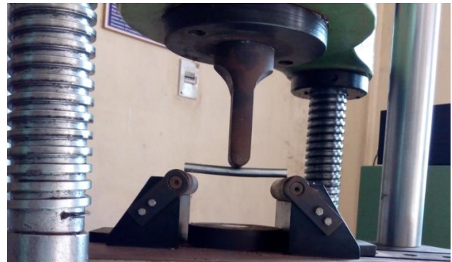
Fig.4.1: Flexural testing setup
