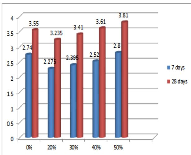
Figure 6.2 Comparison of 7 days and 28 days Split tensile strength of Conventional concrete and other mix
