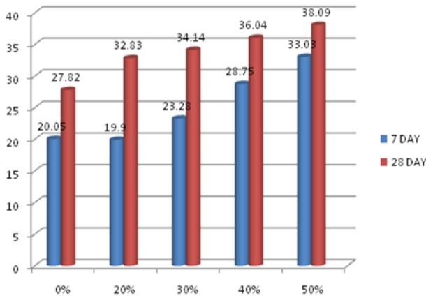
Fig. 6.1 Comparison of 7 days and 28 days compression strength of Conventional concrete and other mix
