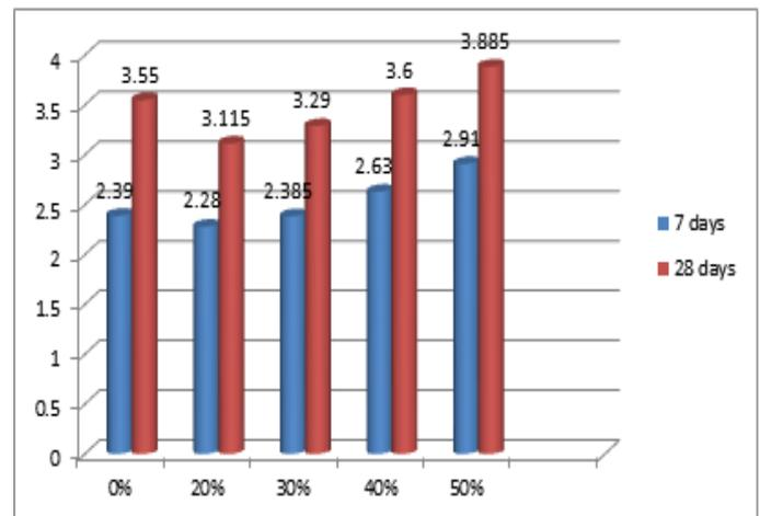
Fig. 6.3 Comparison of 7 days and 28 days Flexural strength of Conventional concrete and other mix
