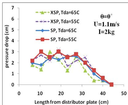
Fig. 2 Pressure drop along the riser height for  $\theta = 0^\circ$  at different temperature
