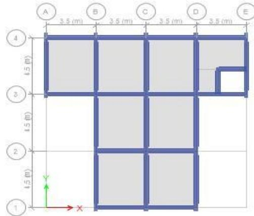
Fig. 4 Plan of asymmetric T shape structure
