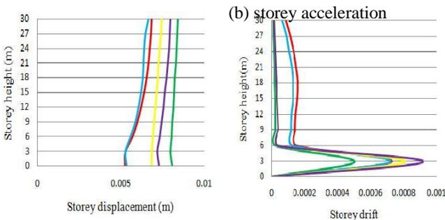
Fig.16 (a) storey displacement (b) Storey drift
