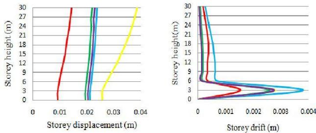
Fig.8 (a) Storey displacement (b) Storey drift
