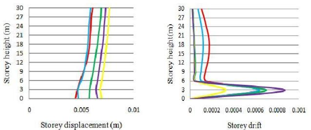
Fig.12 (a) storey displacement (b) Storey drift
