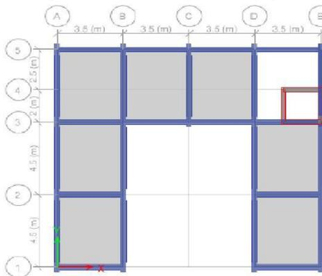
Fig 3: Plan of asymmetric C shape structure
