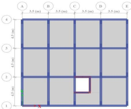
Fig 1: Plan of rectangular base isolated structure
