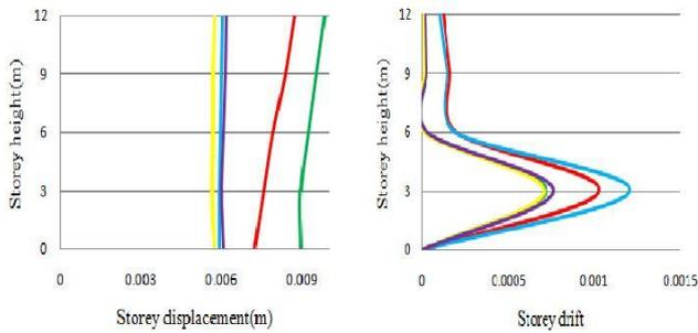
Fig.14(a) storey displacement (b) Storey drift
