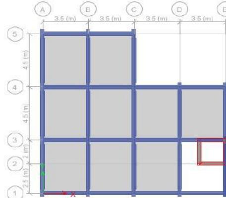
Fig 2 Plan of asymmetric L shape structure
