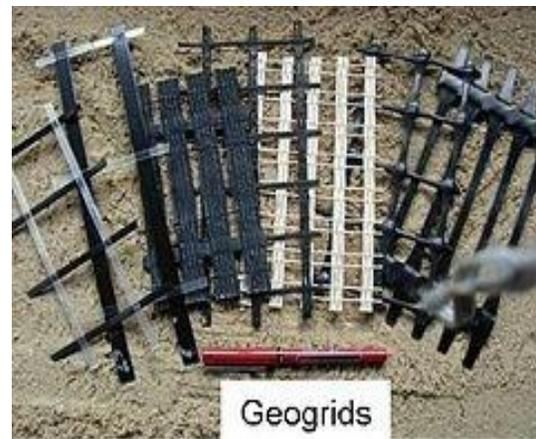
Fig1.1 Different types of geo-grids
