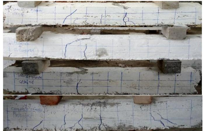
**Fig 4.1 : Crack Pattern of Type A beam specimens**
