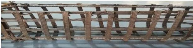
**Fig4.4: Confinement of geo-grid to reinforcement cage.**
