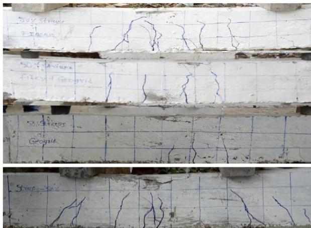
Fig 4.3 : Crack Pattern of Type B beam specimens.
