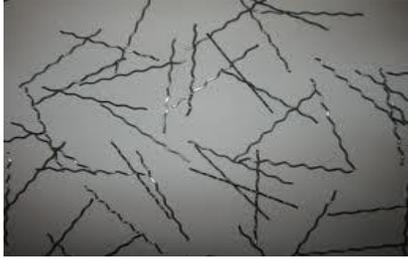
Fig 2.1: Different types of Steel Fibres
