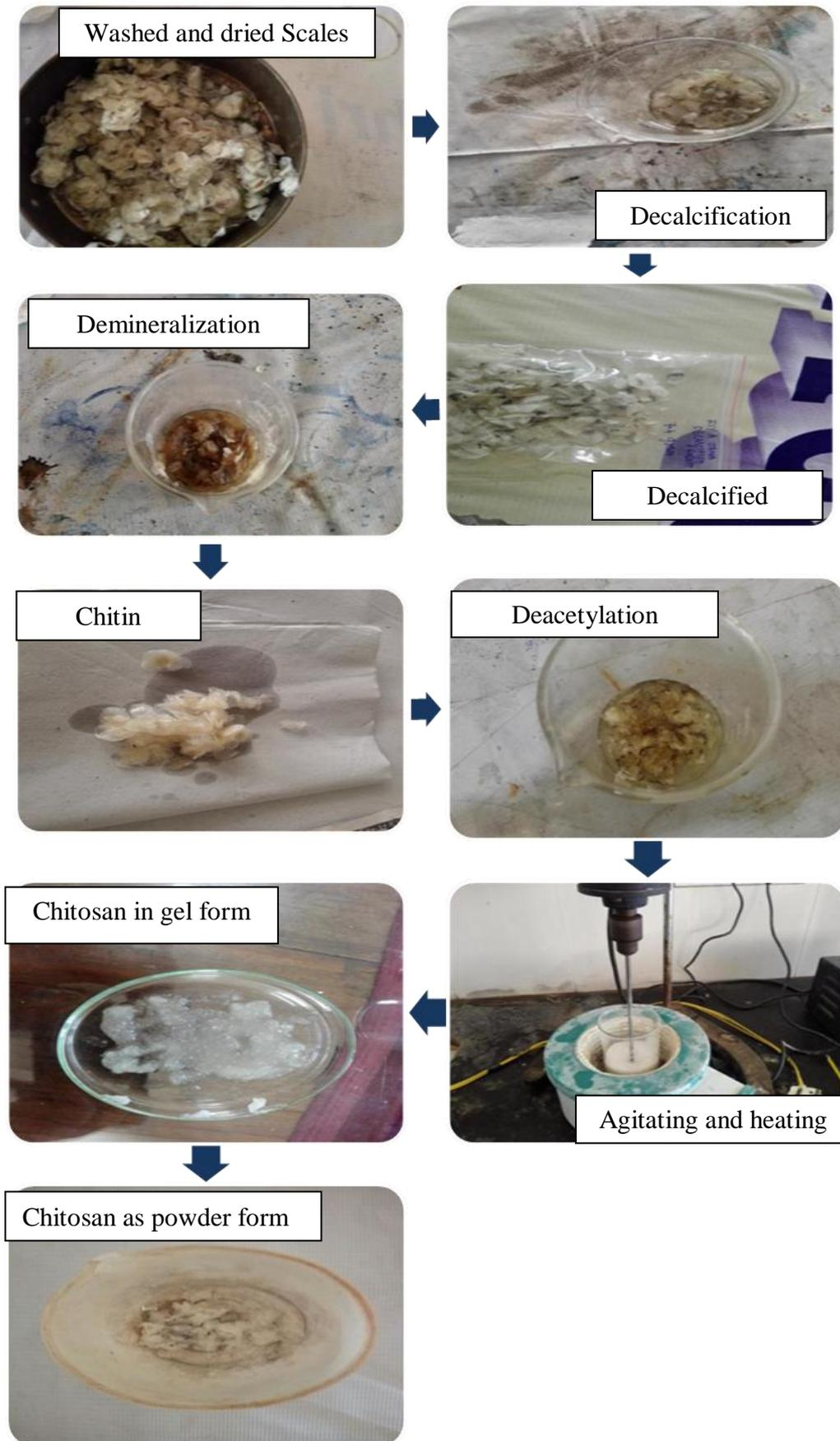
**Figure 3: The photographs of step wise procedure followed in preparation of chitosan using fish scales**
