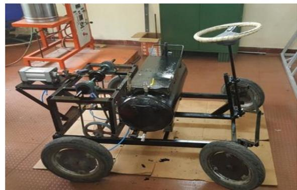
Figure 1. Compressed air vehicle
