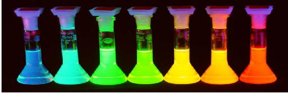
Figure 2: Photoluminescence from CdSe/ZnS (core-shell colloidal) quantum dots of different sizes (~2-6 nm) pumped with the same laser
