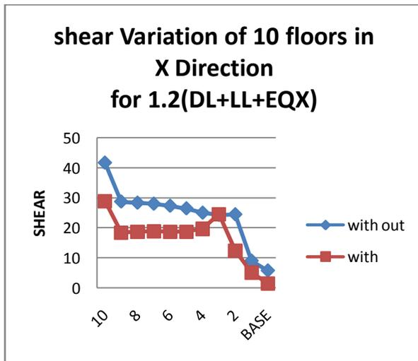
**Graph 4.1 Showing shear variation for 10 floor building in X direction**
