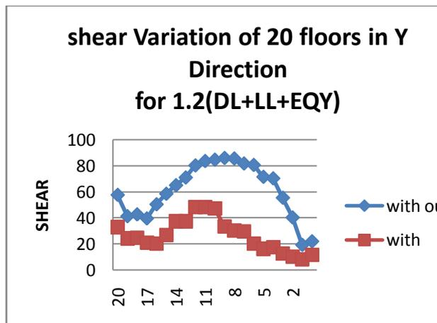
**Graph 4.3 Showing shear variation for 20 floor building in y direction**
