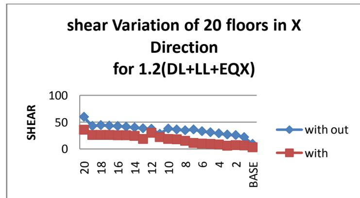
**Graph 4.2 Showing shear variation for 20 floor building in X direction**
