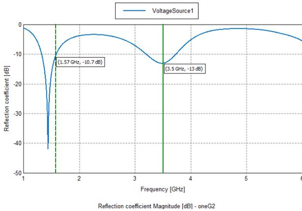
Fig.3. S-parameters curve for dual band hexagonal strip monopole antenna using FEKO
