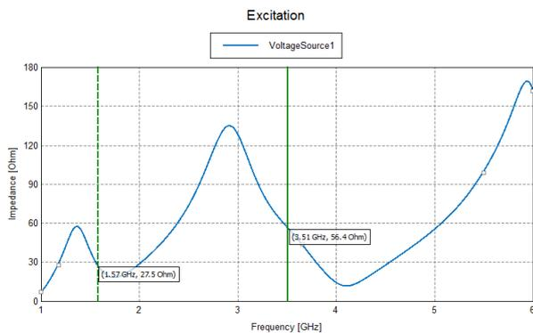
Fig.5. Impedance curve for dual band hexagonal strip monopole antenna using FEKO
