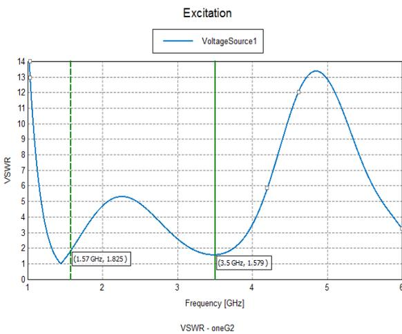
Fig.4. VSWR curve for dual hexagonal strip monopole antenna using FEKO
