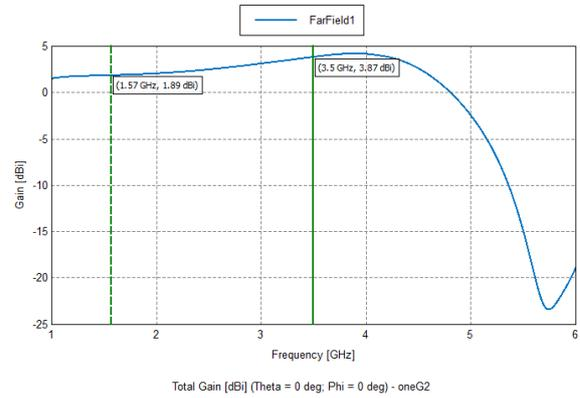
Fig.6. Gain curve for dual band hexagonal strip monopole antenna using FEKO
