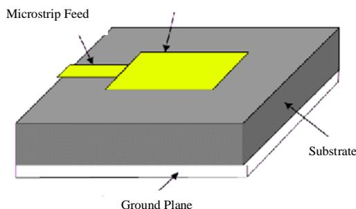
Fig.1. Simple Rectangular Microstrip Patch Antenna
