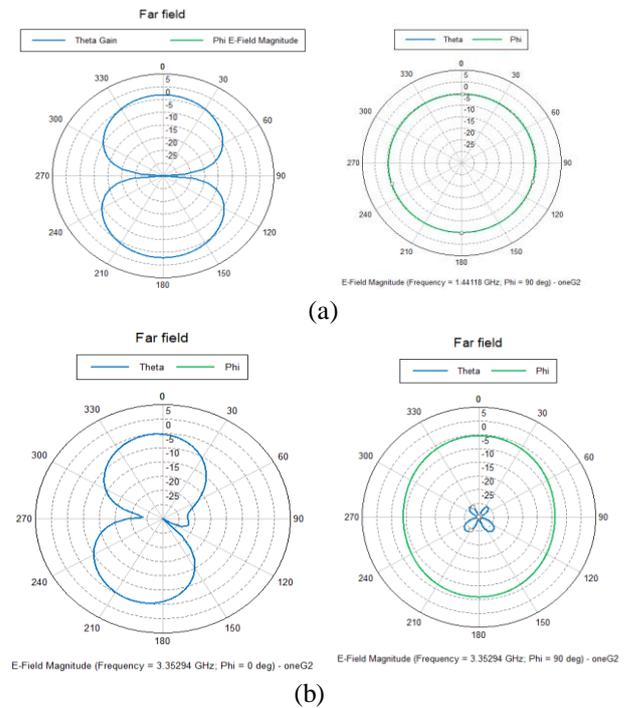
Fig.7. Simulated radiation patterns for dual band hexagonal strip monopole antenna using FEKO
