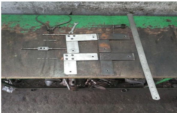
Fig-1.2 Tools and equipment's to complete the Joint.
