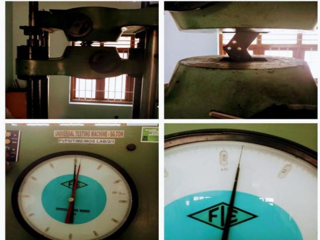
Fig-2.2 Mounting & Loading of Bolted Joint.
