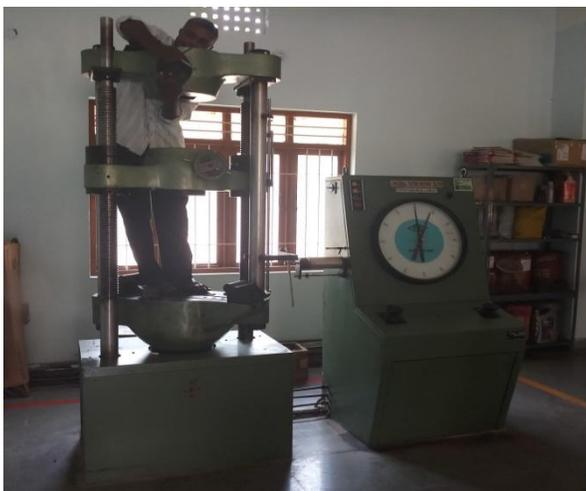
Fig-2.1 Universal Testing Machine (UTM)
