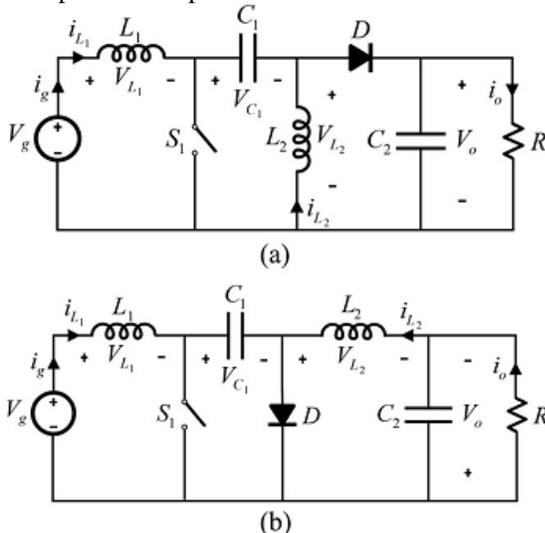
Fig. 2. SEPIC and Cuk converters. (a) SEPIC converter. (b) Cuk converter.
