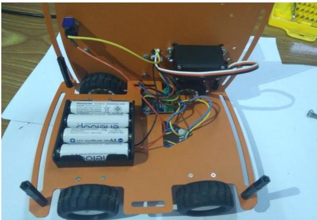
Figure .4. Power and motor driver module
