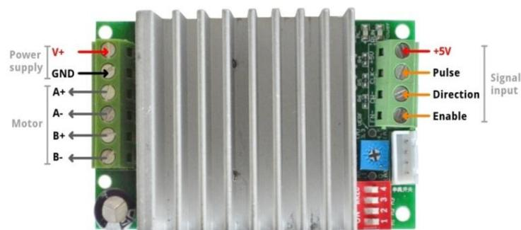
Figure.2 Single Axis TB6600 Stepper Motor Driver IC
