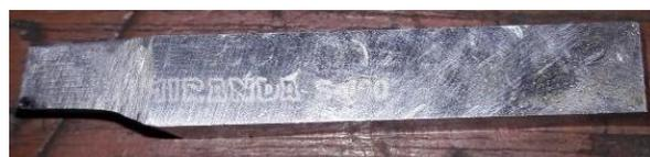
**Fig 3.1 HSS Single Point Cutting Tool**
