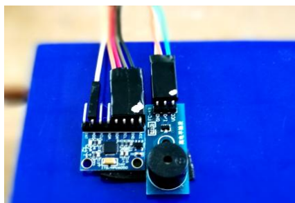
Figure 4. Interfacing with Buzzer Place
