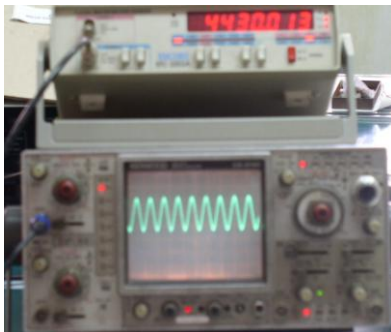
Fig.9. Output Waveforms of Receive Mixer
