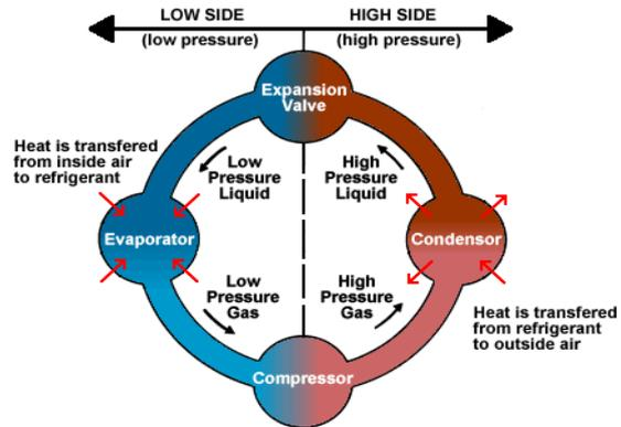
Fig(2) Vapor Compression Refrigeration Cycle
