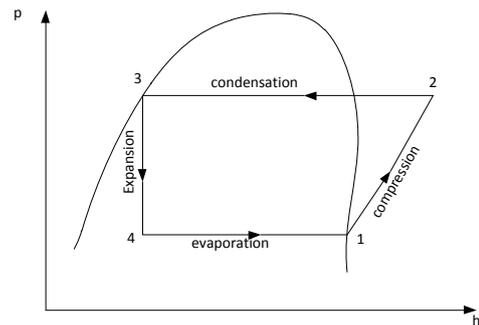
Fig (3) Pressure –Enthalpy diagram (Saturated condition)
