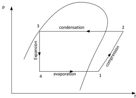
Fig( 4) pressure-enthalpy diagram (superheated condition)
