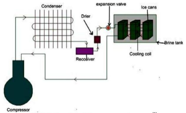
Fig(1) Working principle of vapor compression system
