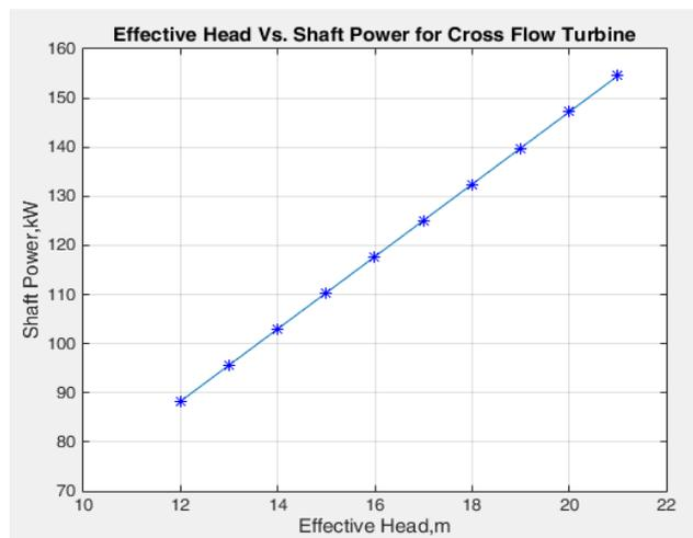
Figure 7. Performance curve of cross flow turbine (shaft power Vs effective head)
