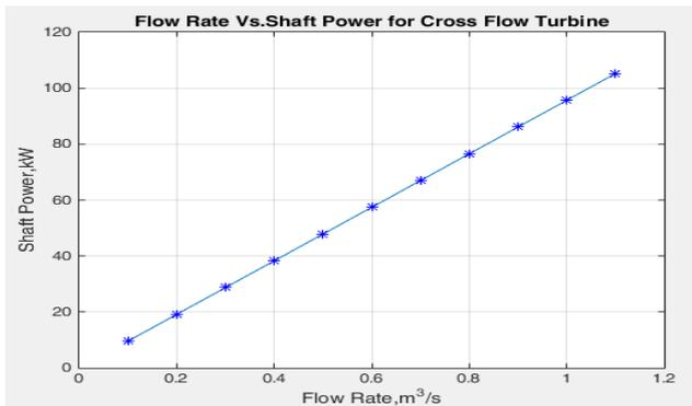
Figure 6. Performance curve of cross flow turbine (shaft power Vs flow rate)
