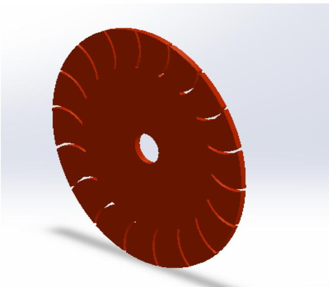
Figure 3. Cross flow turbine runner disc with 3D model
