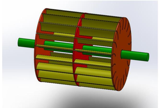
Figure 4. Cross flow turbine rotor
