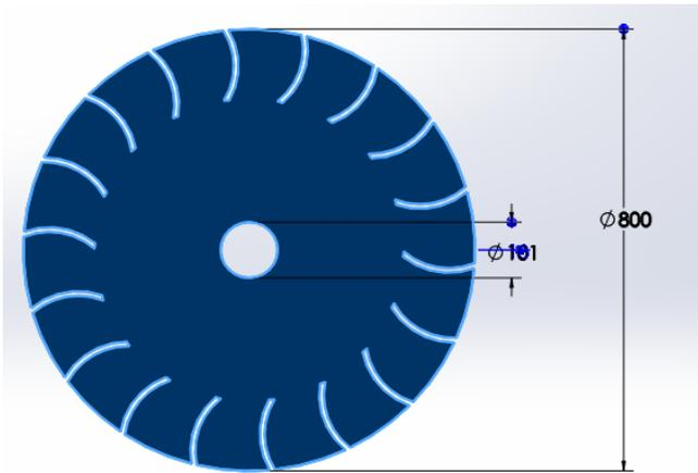
Figure 2. Cross flow turbine runner disc
