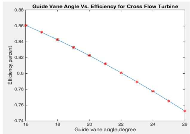
Figure 8. Performance curve of Cross Flow Turbine (Guide Vane Vs Efficiency)
