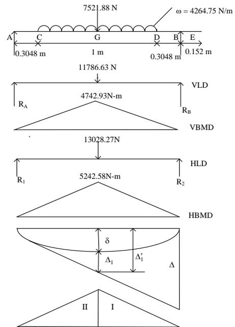
Figure 5. Loading and Bending Moment Diagram
