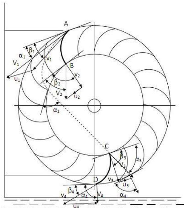
Figure 1. Path of water through turbine
