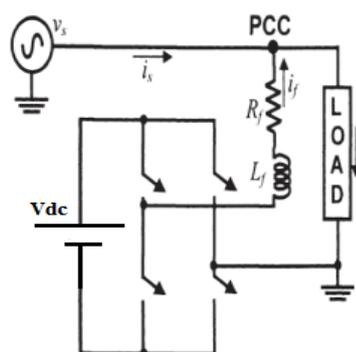
Fig 1 Schematic Diagram of the DSTATCOM Compensation
