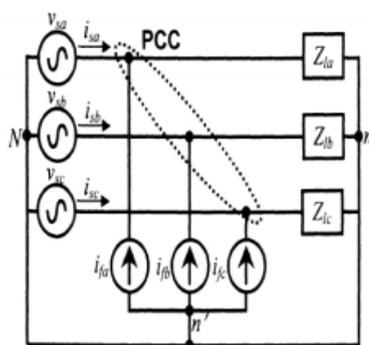
**Fig 2 Three Phase DSTATCOM Compensation Structure**
