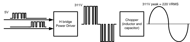
Figure 5. Logic level conversion for Power Driver
