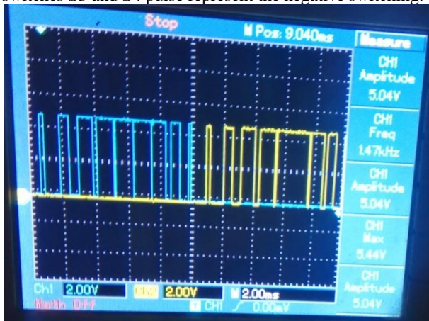
Figure. 14 IR 2110 Gate Driver Output Waveform
