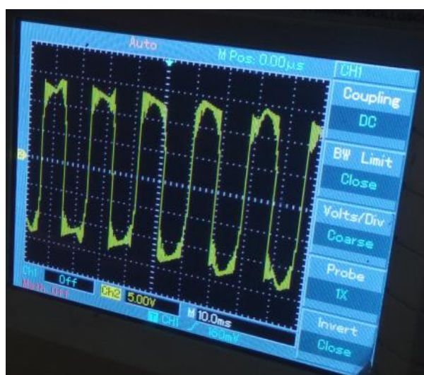
Figure 16. Output waveform of Inverter
