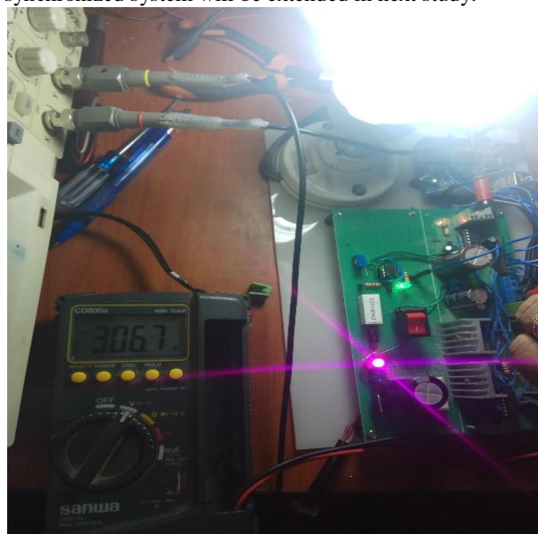
Figure. 18 Output Voltage of the Inverter Circuit when the load is connected
