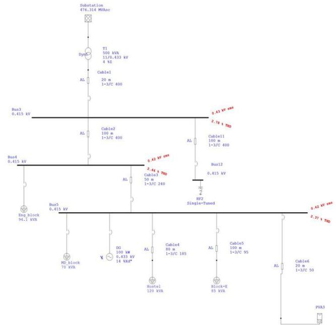
Fig.4 THD for single tuned harmonic filter connected to grid connected PV system
