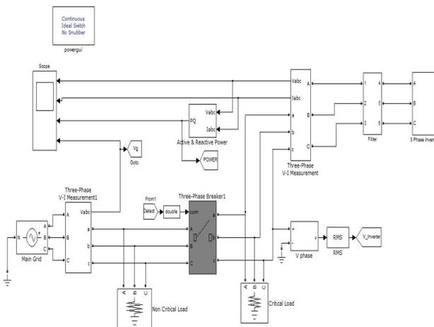
Fig. 4: Proposed Islanding Detection Technique Simulation diagram
