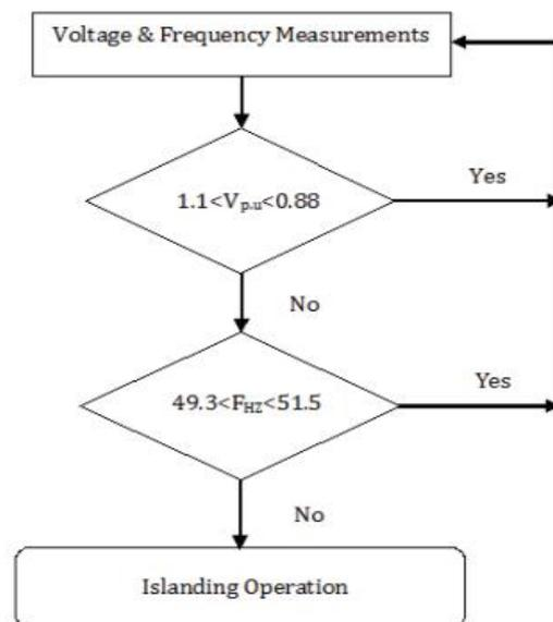
Fig. 3 Flow chart of the Islanding Detection
